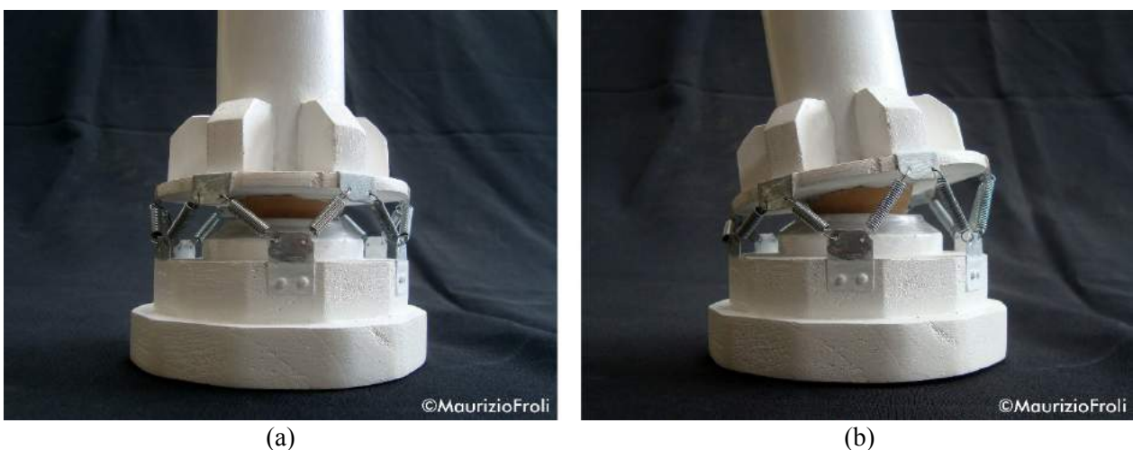
Figure 1 TROCKSISD mock-up: (a) rocking prevented in stick phase, (b) rocking admitted in sliding phase.
