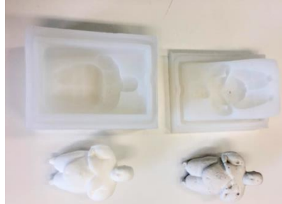
Fig. 1. A two-piece silicone silicone mold used to reproduce the female figurine form Çatalhöyük. Bottom two examples of the fabricated replicas, in resin (left) and gypsum (right).
